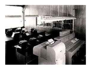
Completed in October 1954, the FACOM 100 was Japan's first relay-type electronic computer.
